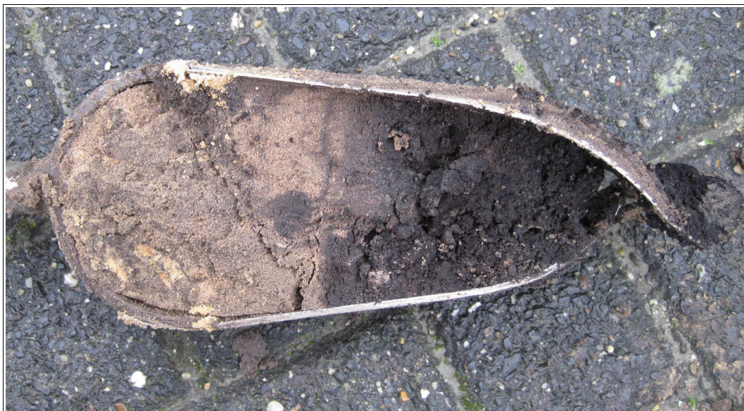
Figuur 10: Westerbork, Zandhoeklaan 7-9: monster boring 6 van 140 tot 150 centimeter. Rechts is veen, links is stuifzand.
